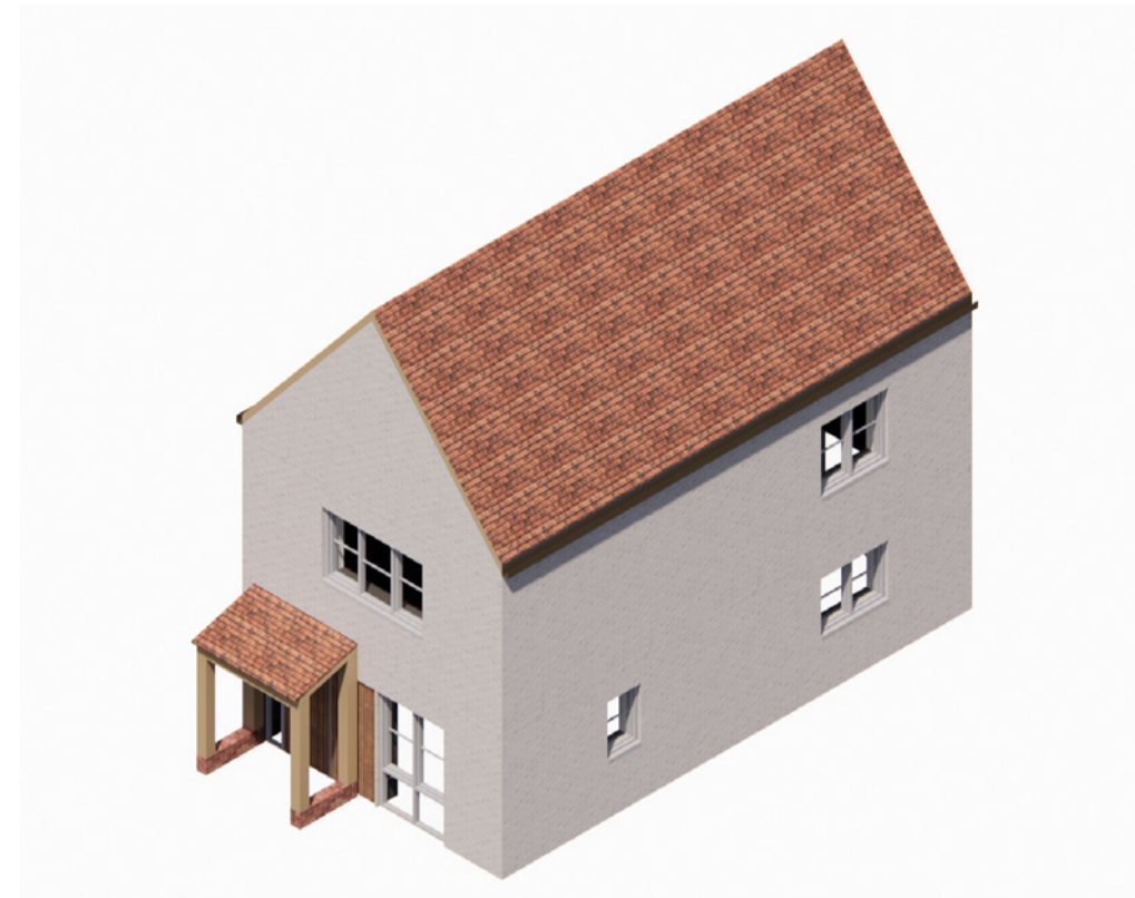
A 2-bedroom house with white painted brick, gable frontage and clay plain tile roof.
